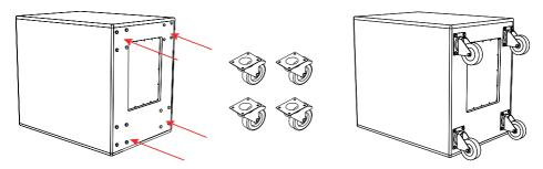
All holes comes with M8 drive-in nut. We suggest to use M8 x 30mm (at least) screws, hexagonal head with washer.
